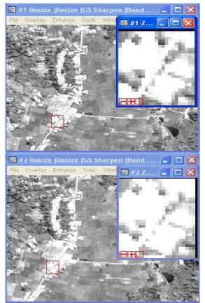
Figure 4: The spectral artifact of Quickbird-PC1/Hyperion fused image bands 18 and 32, respectively
