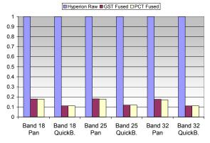
Figure 8: The correlation coefficients between the fused data and the Hyperion raw data (bands 18, 25 & 32)
